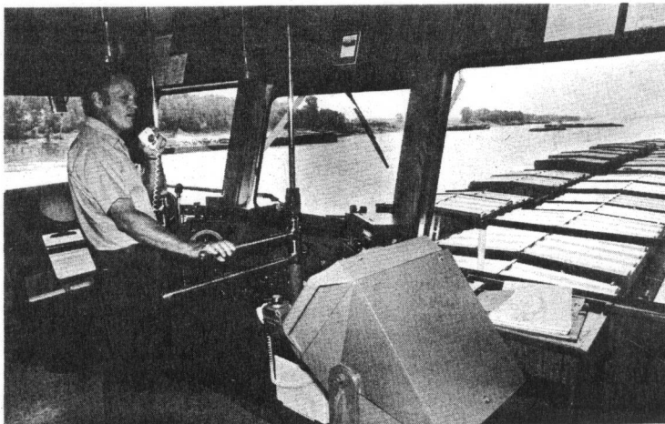
AT THE CONTROLS — Jim Troup mans the controls of the Agnes Mae . In the foreground is one of two radar units, each with its own scanner, which the vessel carries as basic equipment. Jim talks on one of two marine-band FM two-way radios.
