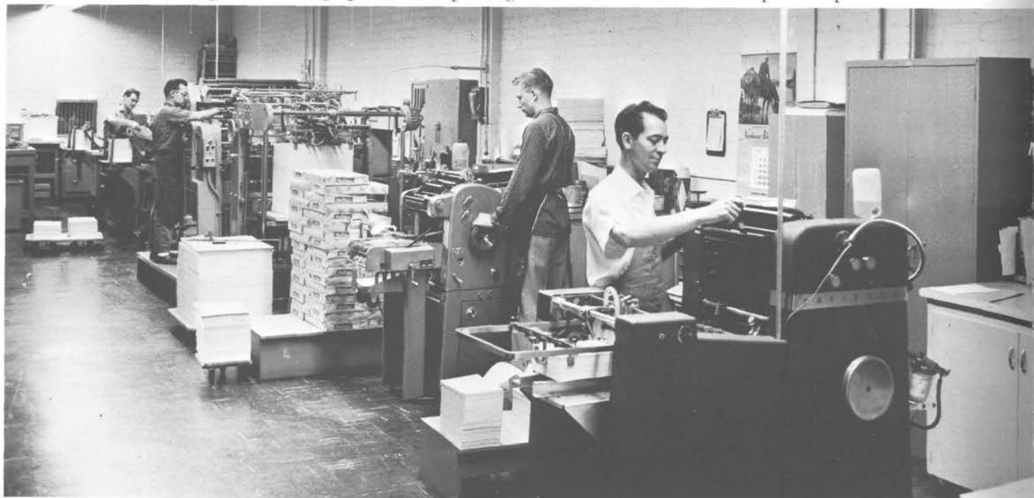
Mr. Winger and Mr. Williams keep everything flowing smoothly through the "Miehle 29." This machine prints over 20,000 pages for the GOOD NEWS every hour.
